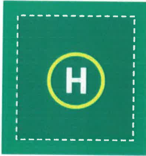
Figure 1 – Secondary HLS: A 1.5 x D FATO with additional 0.25 x D Safety Area (Total area is 2 x D). Also showing 'H', FATO perimeter and 0.5 x D Touchdown/Positioning Markings (TD/PM).
